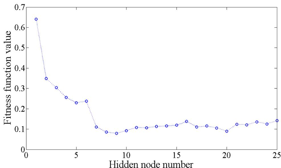
**Figure 10.** Variations in the 5-fold cross-validation data's error levels due to the number of hidden nodes.
