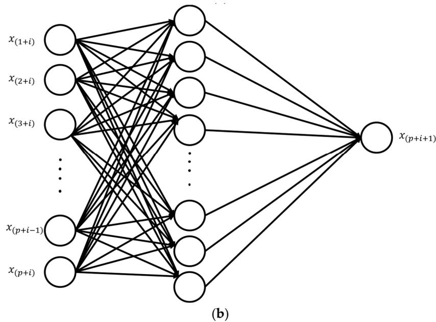
**Figure 2.** (a) The proposed algorithm was used in this study. (b) The structure of the neural network used in this study.
