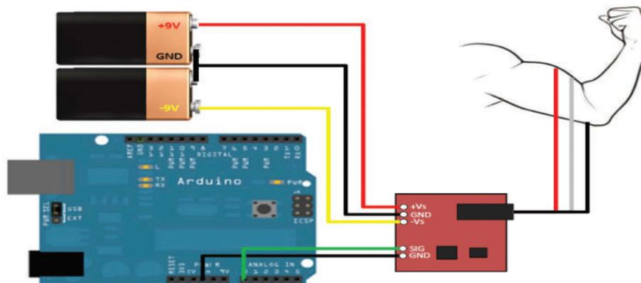
**Figure 2:** Interfacing of EMG sensor with Controller and human arm
