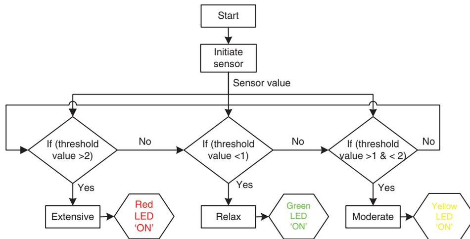
Figure 6: Flow diagram of Muscle fatigue condition based on sensor value
