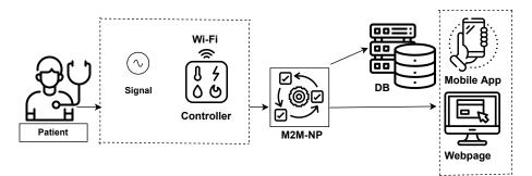
Figure 2. Architecture of an IoT based patient monitoring system.
