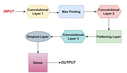
Figure 2. CNN architecture for classification of attacks in IoT Networks.
