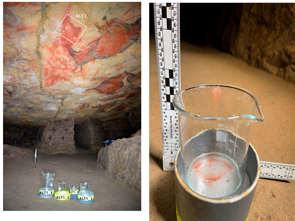
Figure 13. Beakers located perpendicular to the active drip points within the ALT1 control zone. These beakers, designed to capture and quantify the pigment carried by the water droplets, revealed that the visible gap in the ceiling represents only a part of the total pigment lost, as part of the pigment recorded comes from areas bordering the lagoon itself, which access the drip point by migration of the pigment through the sheet of water.
